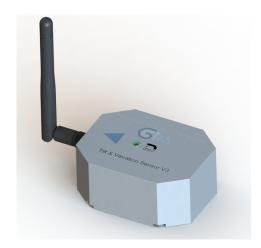
A high precision wireless MEMS vibration sensor with built-in temperature compensation. The sensor has functions similar to an analogue geophone with additional functionality of sending proactive alerts when user defined PPV thresholds are exceeded. The sensor can be remotely configured in the field and upgraded on the fly to a multi-function sensor, with additional modes including 3D orientation,
